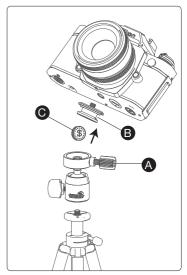
Combining with a tripod and make sure it is firmly. Mount Quick release clip with the camera on the Mounting platform, and screw in Quick release knob. Before shooting, please use Ballhead knob to rotate the camera freely in 360°. Adjust the camera to a proper position and you can start shooting.
